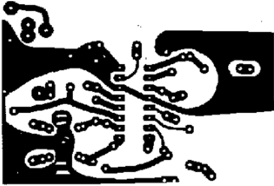
FIGURE 6A. BOTTOM VIEW OF PRINTED CIRCUIT BOARD
