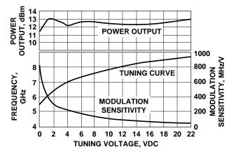
Figure 11. VTO-8650 Power Output, Frequency and Modulation Sensitivity vs. Tuning Voltage.
