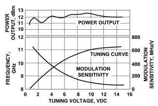
Figure 14. VTO-8950 Power Output, Frequency and Modulation Sensitivity vs. Tuning Voltage.
