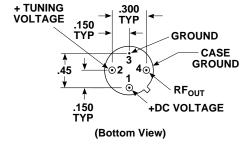
Figure 15. TO-8 Test Fixture.
