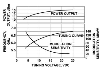
Figure 10. VTO-8580 Power Output, Frequency and Modulation Sensitivity vs. Tuning Voltage.
