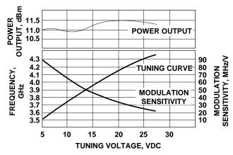
Figure 8. VTO-8360 Power Output, Frequency and Modulation Sensitivity vs. Tuning Voltage.
