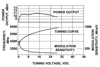
Figure 9. VTO-8430 Power Output, Frequency and Modulation Sensitivity vs. Tuning Voltage.
