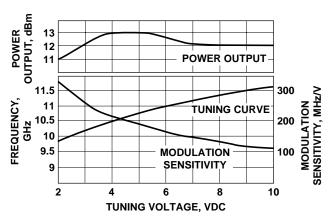
Figure 15. VTO-810750 Power Output, Frequency and Modulation Sensitivity vs. Tuning Voltage.
