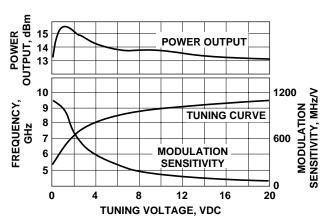
Figure 12. VTO-8810 Power Output, Frequency and Modulation Sensitivity vs. Tuning Voltage.
